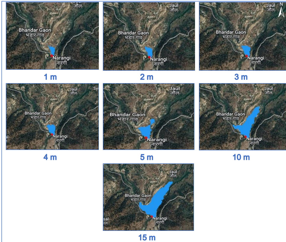
Fig. 5.15. Water spread area at the outlet of the catchment based on ALOSPALSAR (12.5 m) DEM at different dam heights.
